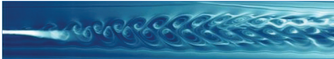
Vortex shedding at a laminar wind inflow
