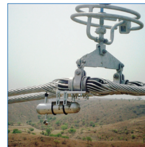
Field measurement with recorder at a HSU clamp
