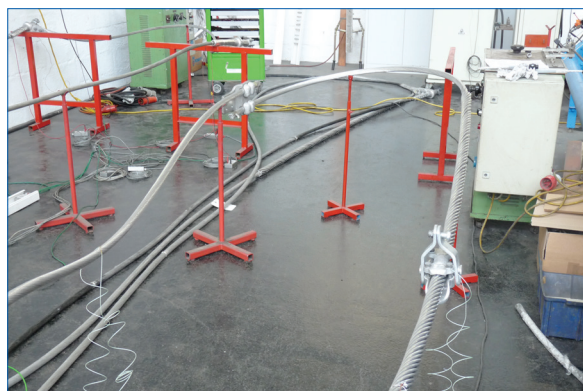
Heat cycle test with suspension clamps for high-temperature conductors
