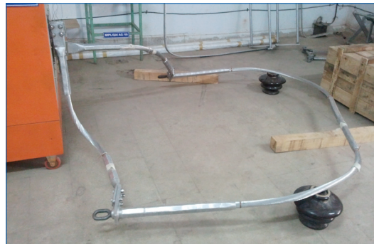
Ageing test with compression dead end clamps for high-temperature carrying conductors in the laboratory
