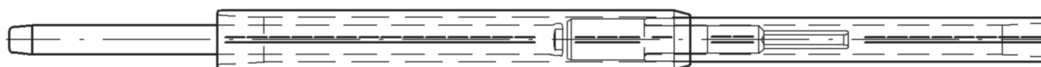
Compression joint for the connection of a hollow conductor with an Aluminium-Steel conductor
