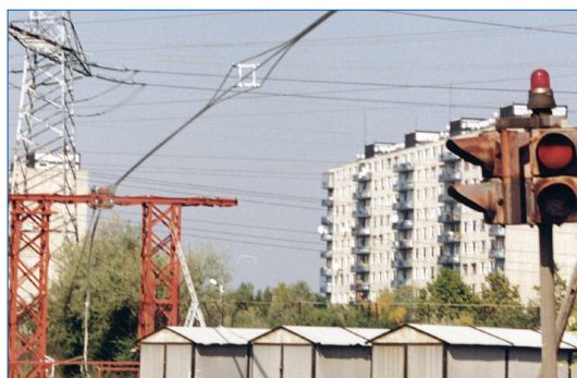
Short circuit test made on spacer dampers
